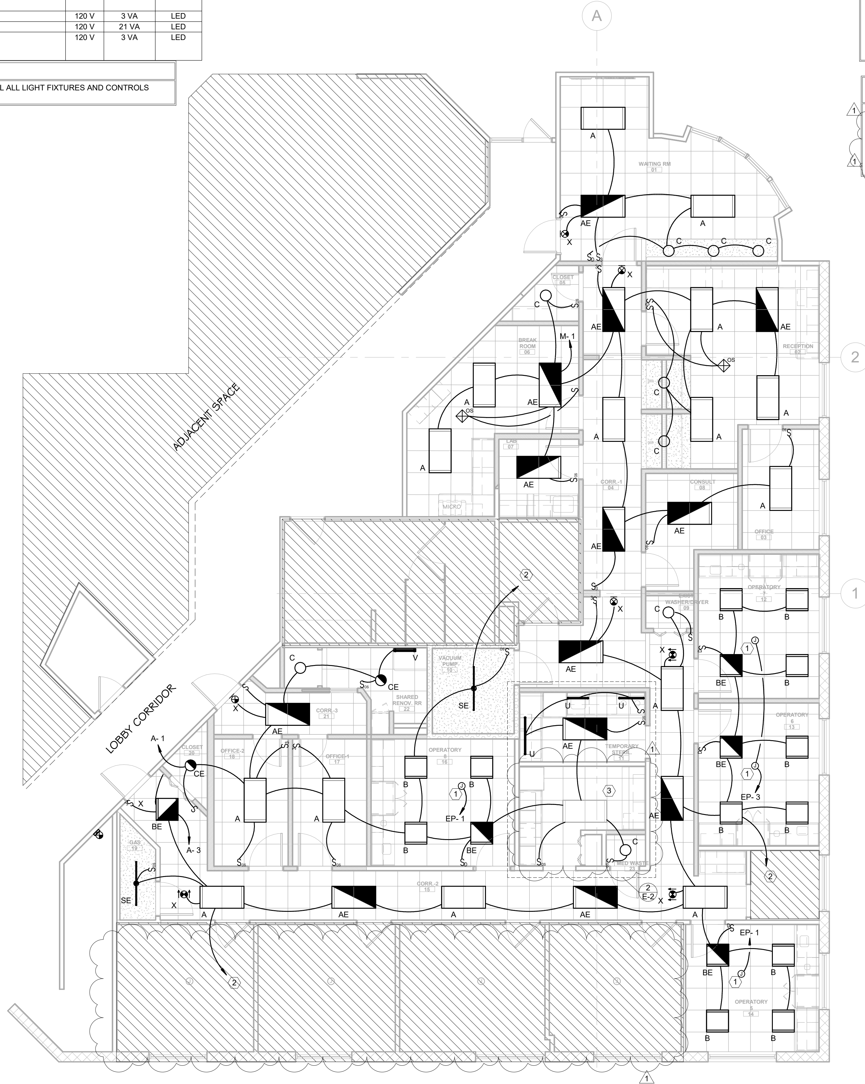
1 FLOOR PLAN - LIGHTING E-2 3/16" = 1'-0"
